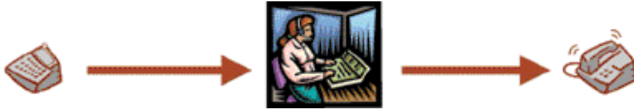
Figure 2.23. The relay service user's call from a textphone to a voice phone goes automatically through the Relay Service for Text Telephony.
